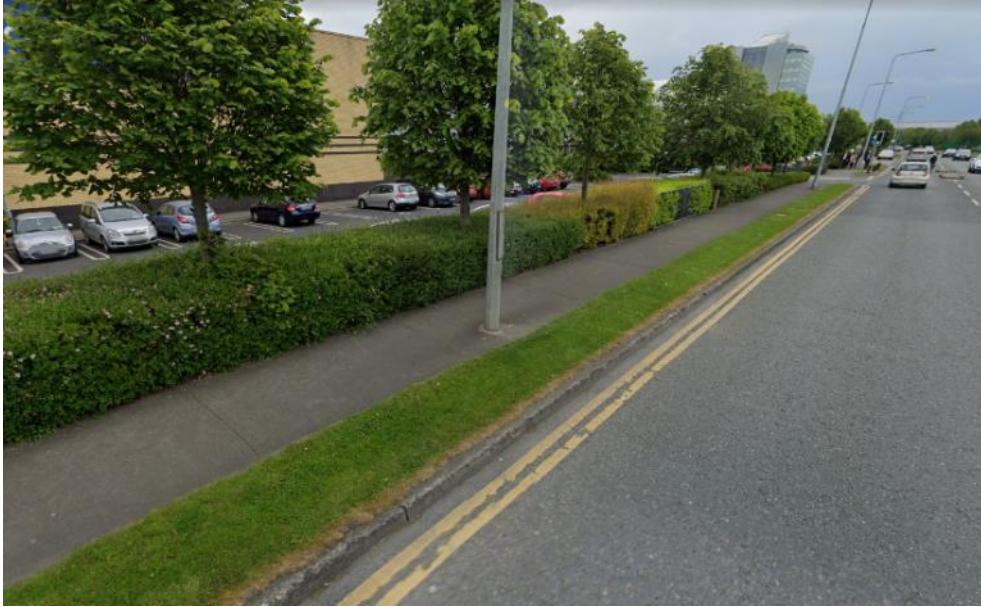
Figure 4: Effective width of footpath reduced due to lamppost placement. – Blanchardstown Shopping Centre
